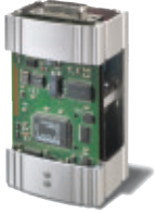
An insight into a compact drive electronics system with a small output (Pfeiffer Vacuum GmbH)
