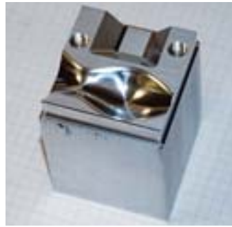
Machined free-form surface contour: the precision cutting with the Servoone means no polishing stage is required.
