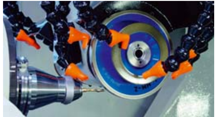
Manufacture of carbide-tipped cutters: the high dynamism of the Servoone help increase the machine's speed and cycle rate Picture: Andron
